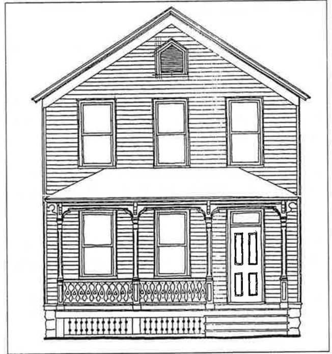
Wood frame house showing types of trim
